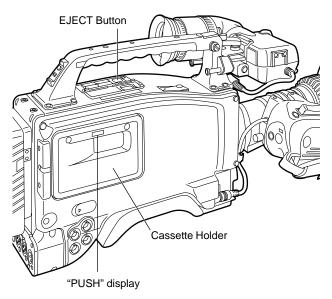
3 Check there is no slack in the tape, insert the cassette, then press the "PUSH" display on the cassette holder to close the cassette holder firmly.
